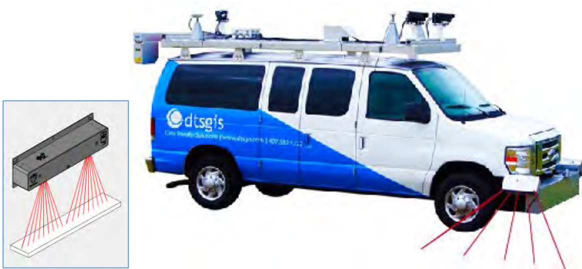
Figure 1 - Laser Profiler and Van Survey Equipment
