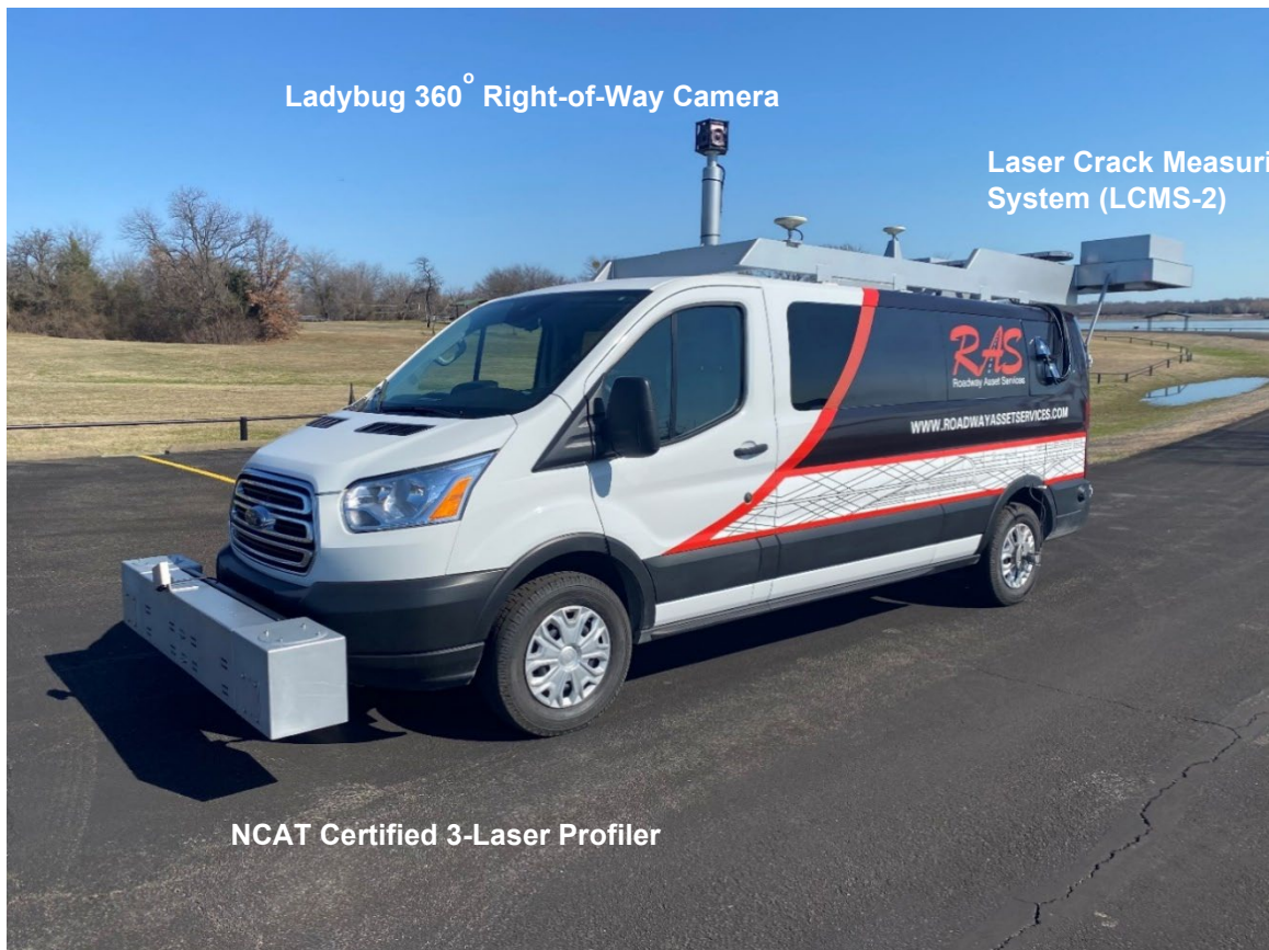
Figure 1 - Laser Profiler and Van Survey Equipment
