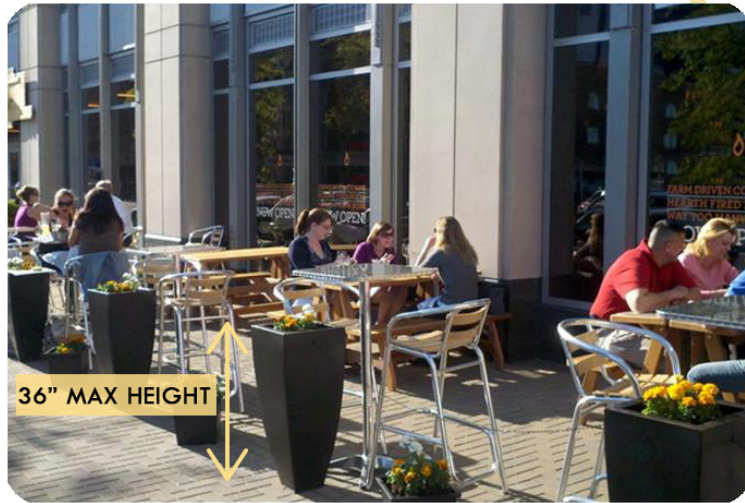
Figure 4. Max height of barriers is 36 inches.
