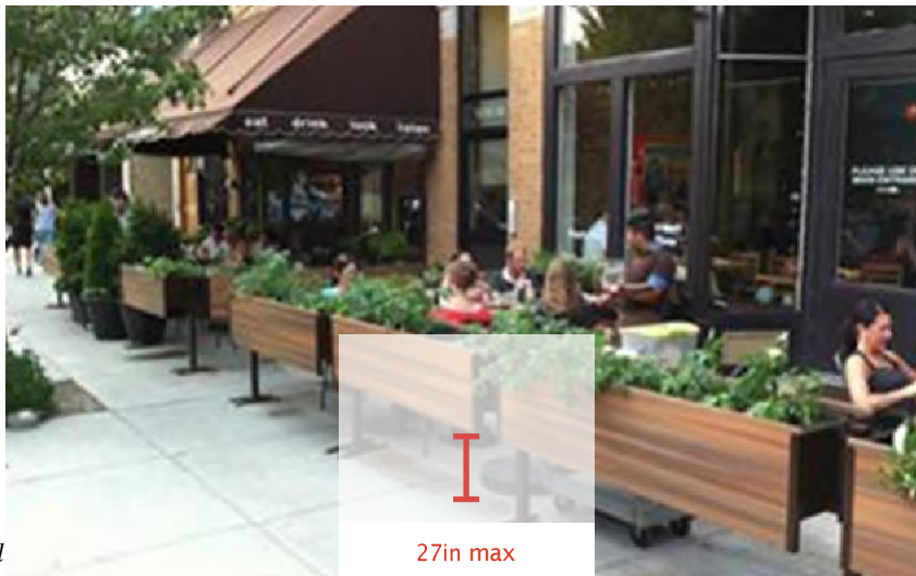
FIGURE 8.3 MAXIMUM HEIGHT ABOVE SIDEWALK SURFACE
