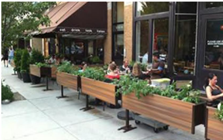
FIGURE 7.1 PLANTERS USED AS FREESTANDING BARRIERS
