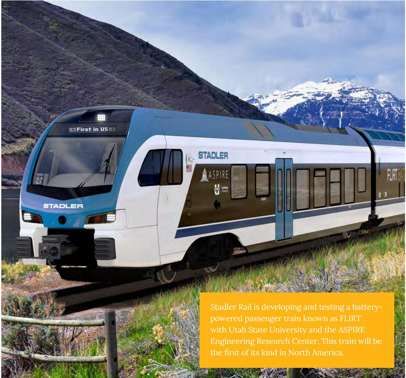
Stadler Rail is developing and testing a battery-powered passenger train known as FLIRT with Utah State University and the ASPIRE Engineering Research Center. This train will be the first of its kind in North America.
