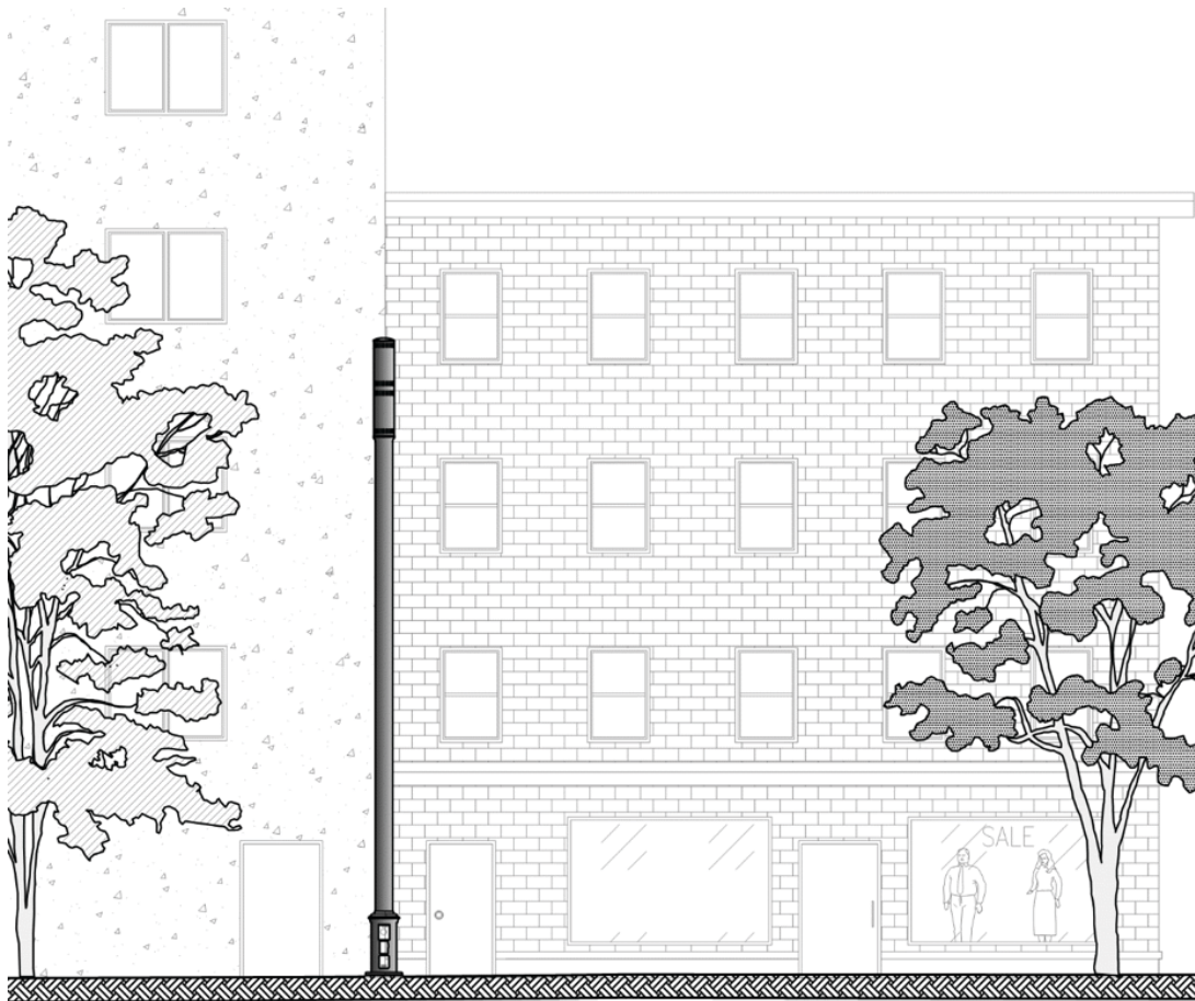
Figure 5-9: Small Cell in Commercial Area
