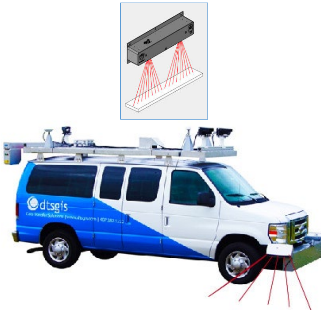
Figure 1 - Laser Profiler and Van Survey Equipment
