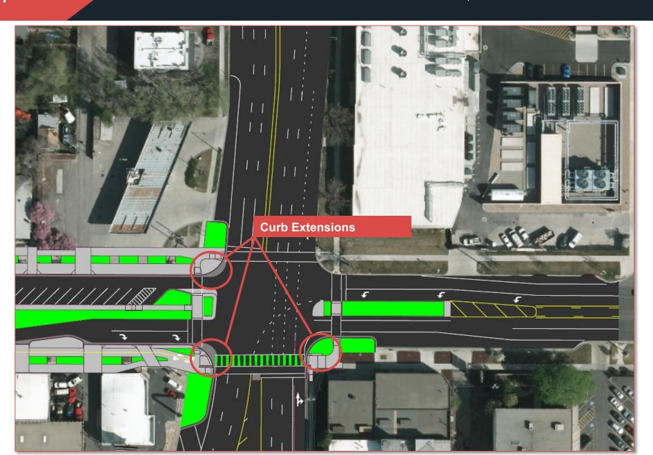
**Parking Repurposed to Accommodate** a NB the Lane Merge Parking Repurposed to Accommodate the Trail and Left-Turn Lane
