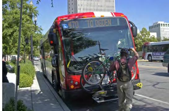
UTA buses are equipped with bicycle racks with enough room for two bicycles.
