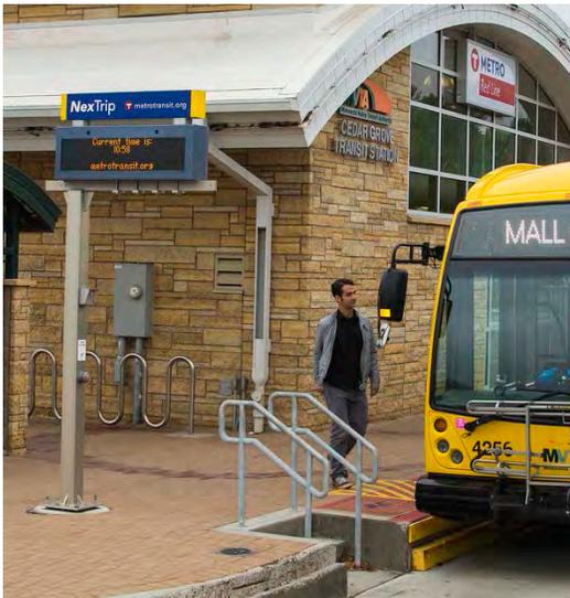
Bus stop accessibility features include audible “next bus” announcements, activated using a button on the stop pole, and a level-boarding platform with tactile strips.
