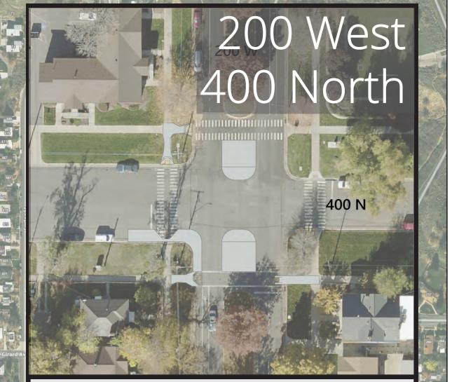
Curb extensions: slow vehicle speeds, reduce pedestrian exposure, ADA compliant
