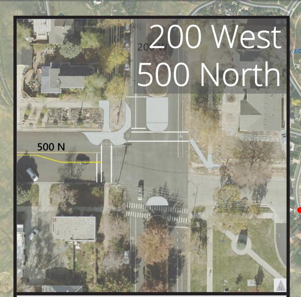
Curb extensions: slow vehicle speeds, reduce pedestrian exposure, ADA compliant,
