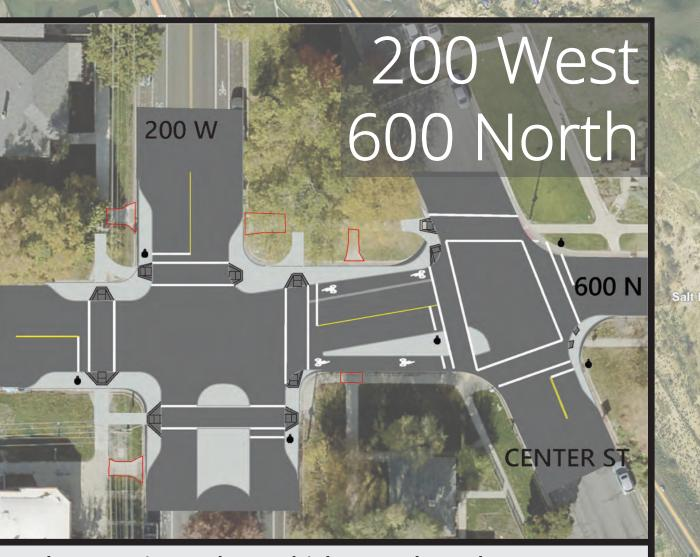
Curb extensions: slow vehicle speeds, reduce pedestrian exposure, ADA compliant, coherent walking paths
