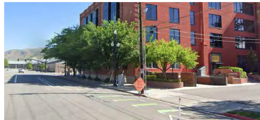
Photos (top to bottom): Typical application of green conflict markings (NACTO, 2019). Example of green conflict markings on 200 W in Salt Lake City.
